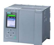
SIMATIC S7-1500, CPU 1518-4 PN/DP, central processing unit with 6 MB work memory for program and 60 MB for data, 1st interface: PROFINET IRT with 2-port switch, 2nd interface: PROFINET RT, 3rd interface: Ethernet, 4th interface: PROFIBUS, 1 ns bit-performance, SIMATIC Memory Card required
